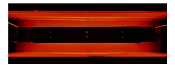
The photo below is a thermal image obtained when a heat-resistant brick was irradiated from a distance of 30 mm.
