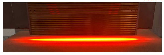
HLH-55W/f25/L280 from a rated focal length of 25mm irradiates firebricks.
