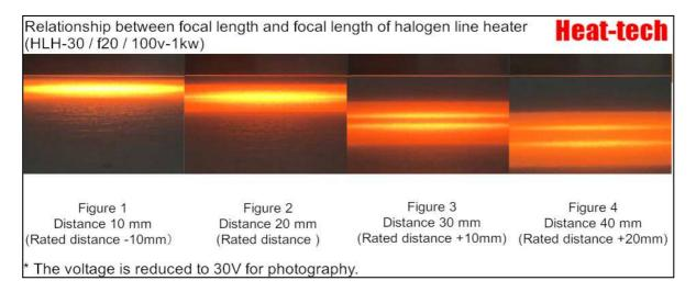
If HLH-30 is separated from a focal length (20mm), it can also perform heating which gave width. Irradiation intensity is even, but the temperature of the center of the higher heat of the peripheral portion is run away.
