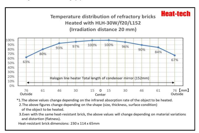
From the thermal image, divide the 152 mm area of the condenser mirror of the halogen line heater into 10 areas, divide the maximum temperature of each divided area by the maximum temperature of the entire area, and quantify the temperature distribution of the heat-resistant bricks.
