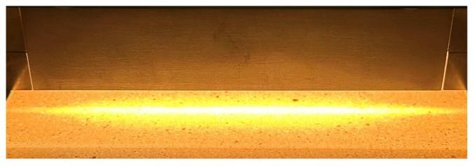
Refractory bricks are irradiated with HLH-30W/f30/L152 from a rated distance of 20mm.
