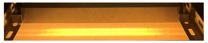
HLH-35W/f∞/L316 irradiates refractory bricks from a distance of 30mm.
