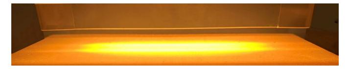
HLH-50W/f∞/L280 irradiates refractory bricks at a distance of 30mm.
