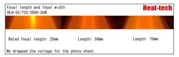
When move away from the rated focal length (25 mm), user can also heat with a certain width. Although the irradiation intensity is uniform, the temperature in the center is high because heat escapes from the periphery.
