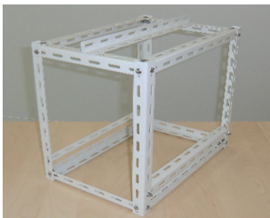
【 Cubic Test Stand for middle & large size heater 】
