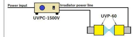
[Usage example: cold cathode UV lamp control]
